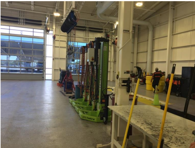
Portable lifts in maintenance bay.
